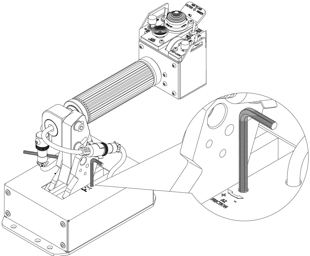
Using an allen wrench to turn the screw for damping force adjustment. CW for increase damping, CCW for reduce damping force.
